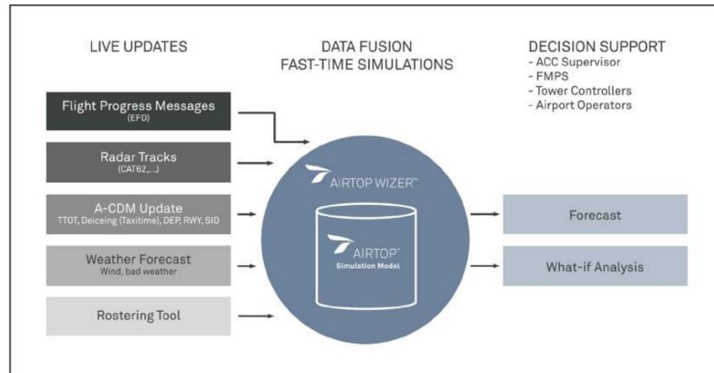
WIZer can model the full operational environment of any ACC or group of ACCs. It provides complexity and controller workload measurements for all types of sector (e.g. en-route sectors, TMAs, etc.), or for tower controllers, and provides ways to manage this complexity and workload. The workload and complexity model is specified using a GUI within the WIZer application which allows the WIZer administrator to modify, parameterize or customize the model.
